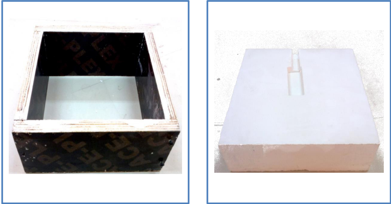
Figure (3-7): Pictures of mould preparation and the mould prepared for a bar sample.
